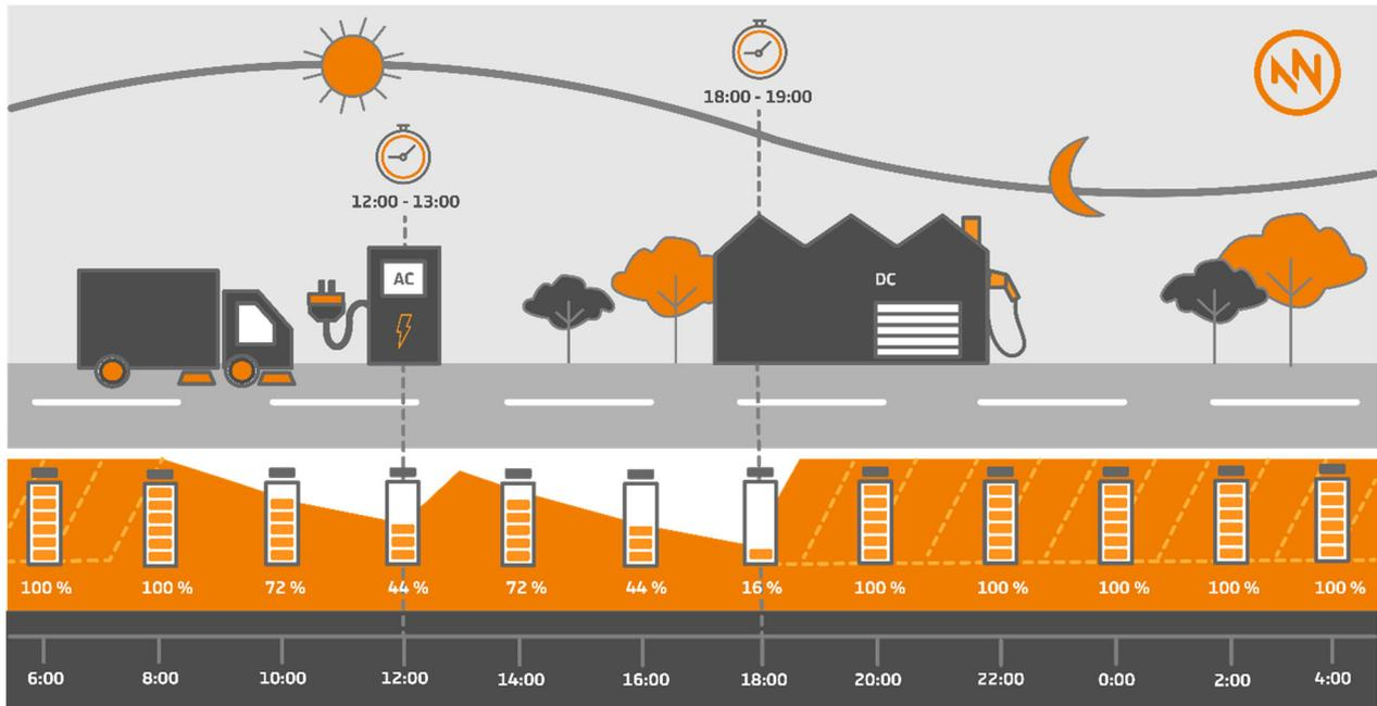
In the first case we consider an electrically powered municipal vehicle used for street cleaning. Characteristic for the daily work are not long distances to be covered - but a permanent use over the shift operation. The municipal vehicle has a battery with a total capacity of 50 kWh.
